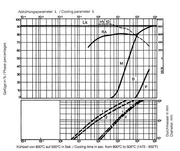
A....Austenite B....Bainite K....Carbide P....Perlite M....Martensite RA...Retained Austenite
